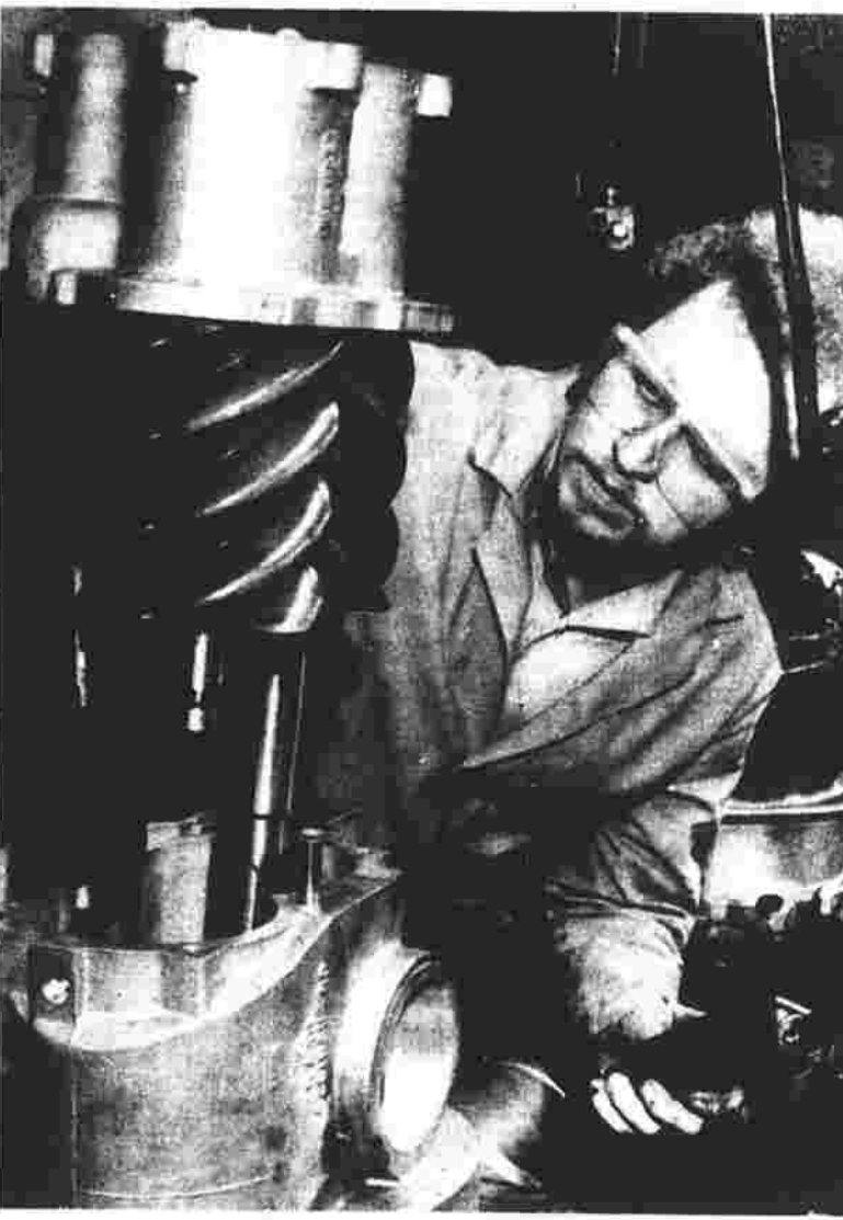
A pair of helical axial rotors — the "heart" of an advanced generation of rotary screw compressors — is lowered into its housing at the Dunham-Bush manufacturing plant in West Hartford. The company builds the unit for commercial and industrial air conditioning and refrigeration. The rotors which never touch, being separated by a thin film of oil, take the place of pistons and crankshafts in conventional reciprocating compressors. Dunham-Bush is one of the Signal Companies. (UPI photo)
